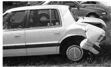
Figure 19: Single photograph used for speed/crush estimate.
