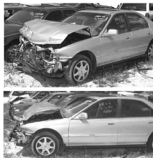
Figures 20a and 20b: Two photographs used together for one crush estimation exercise.
